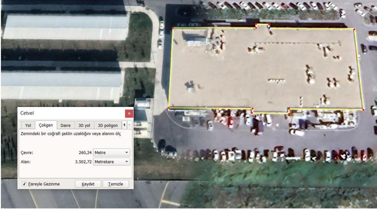
**Figure 10.** Roof group 7 and its polygon area measurement
