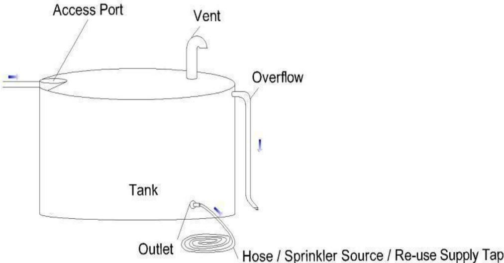
**Figure 15.** The tank and its associated components (Müftüoğlu, 2024)
