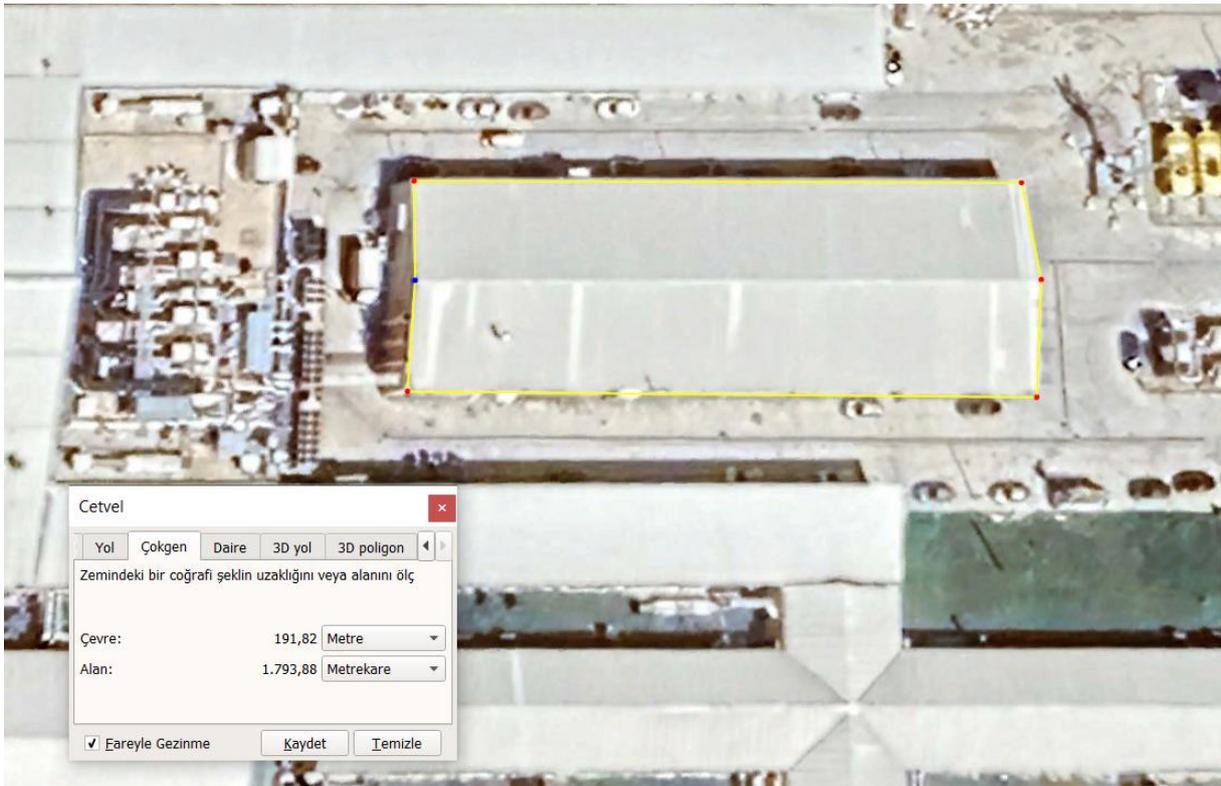
**Figure 9.** Roof group 6 and its polygon area measurement
