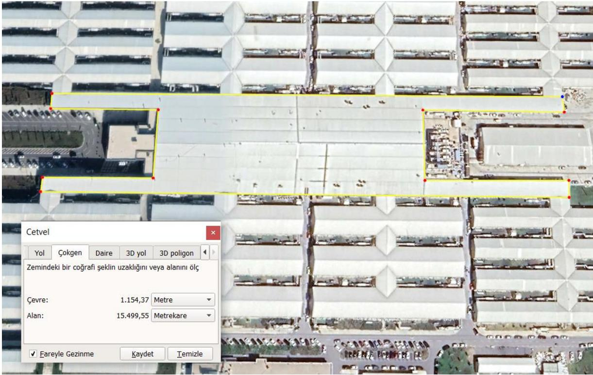
**Figure 8.** Roof group 5 and its polygon area measurement
