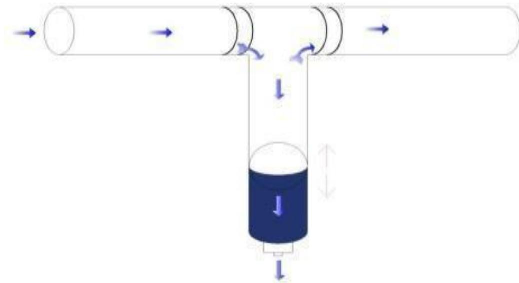
**Figure 14.** The first flush diverter system (Müftüoğlu, 2024)
