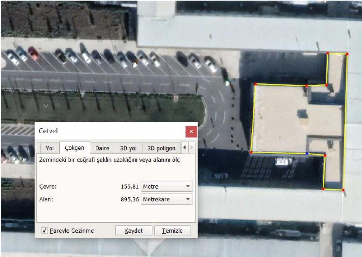
**Figure 11.** Roof group 8 and its polygon area measurement
