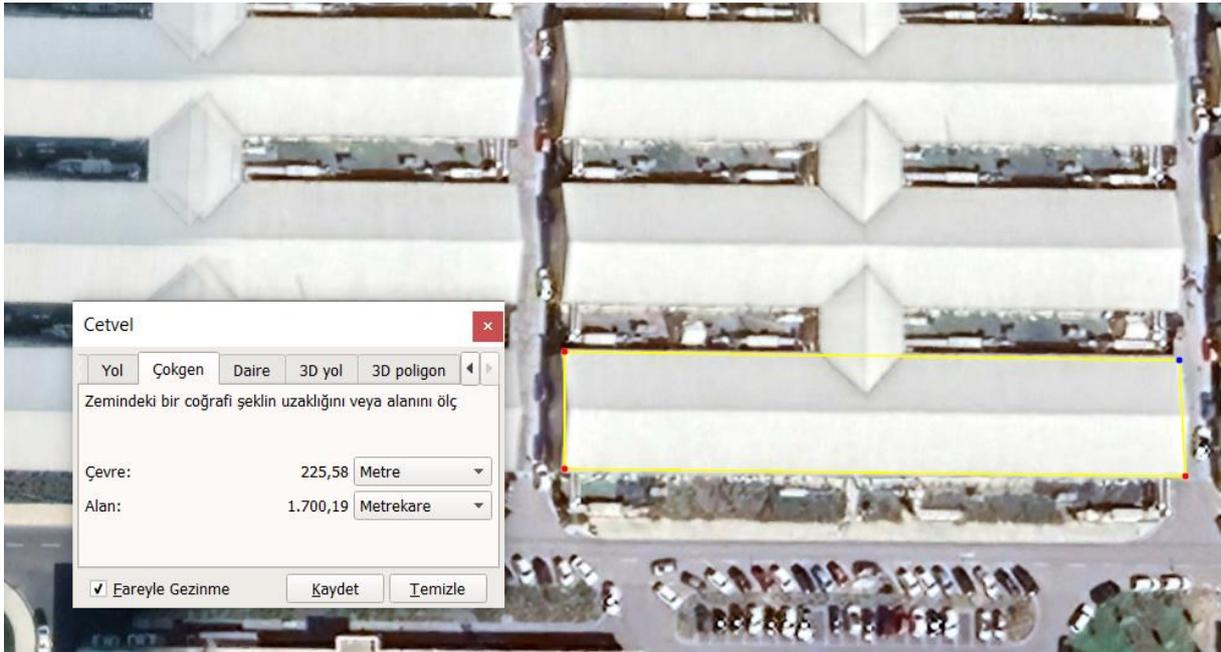
**Figure 7.** Roof group 4 and its polygon area measurement
