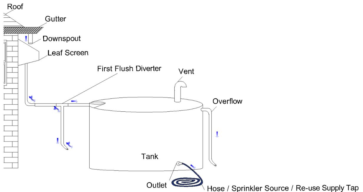
**Figure 12.** Fundamental RWH components (Muftuoglu and Oral, 2024)
